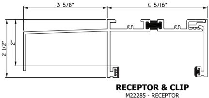
M22285 - RECEPTOR M17378 - CLIP BPN-4189 - RECEPTOR W.S. BPN-9159 - CLIP W.S.
