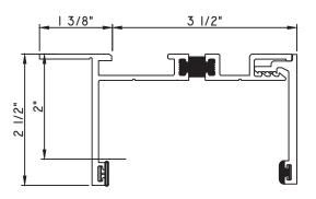
RECEPTOR & CLIP M17376 - RECEPTOR M18140 - CLIP BPN-4189 - RECEPTOR W.S. BPN-9159 - CLIP W.S.
