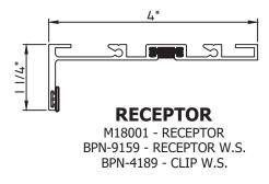
MUST BE USED WITH SUBSILL: M23133 **INSTALL TYPE:** PREASSEMBLED OR SQUARE CUT IN FIELD
